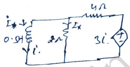
(b) Find v(t) for t > 0 for the circuit given below:
